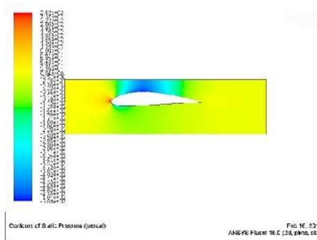
Figure 6: Contour of Static Pressure of NACA 4415
